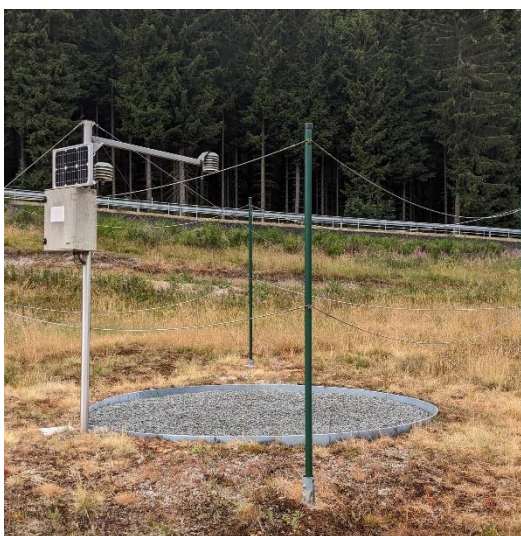
Fig. 2 Automatic snow station – snow pillow type
