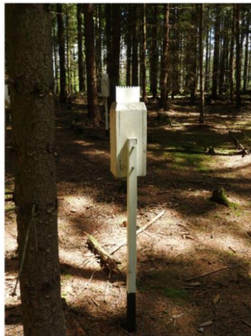
Fig. 12 “Throughfall” sampling, forest stream catchment area of the Košetice observatory (photo: J. Svobodová)
