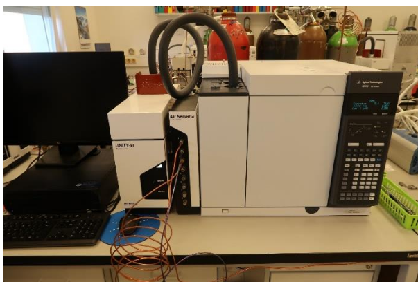
Fig. 13 GCMS analyser for determination of volatile organic compounds (VOCs) collected in canisters (Photo: CQL Prague Libuš)
