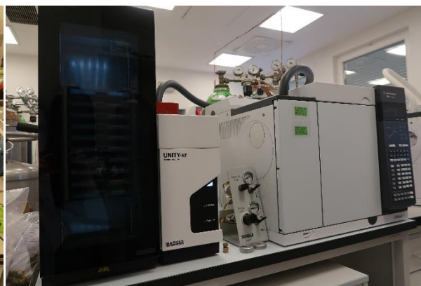
Fig. 14 Gas chromatograph for determination of benzene from sorption tubes (Photo: CQL Prague Libuš)
