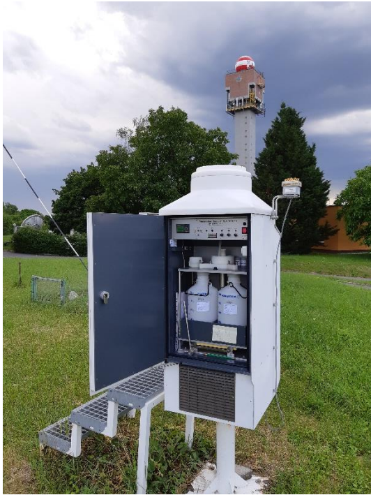
Fig. 17 Automated “wet-only” sampler, Prague-Libuš station (Photo: E. Svobodová)
