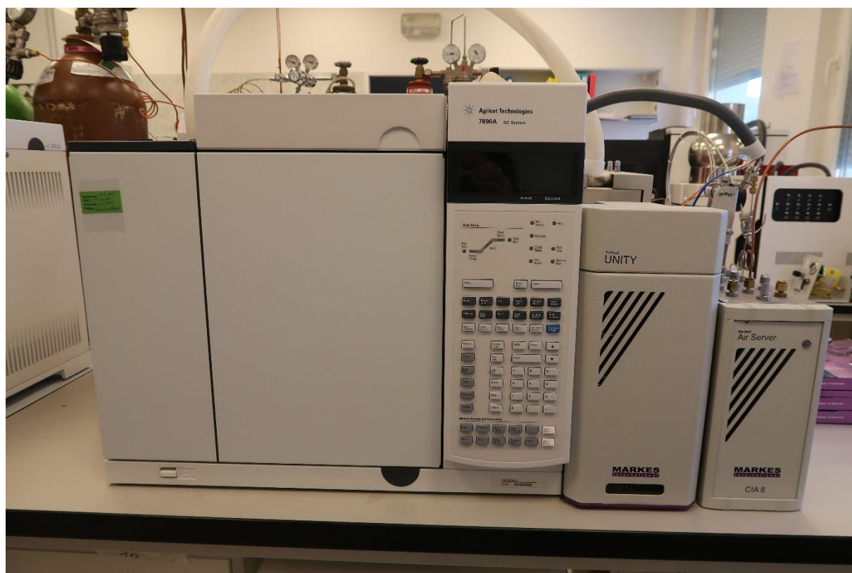
Fig. 11 Gas chromatograph with FID detector for determination of volatile organic compounds (VOCs) in outdoor air (Photo: CQL Prague Libuš)
