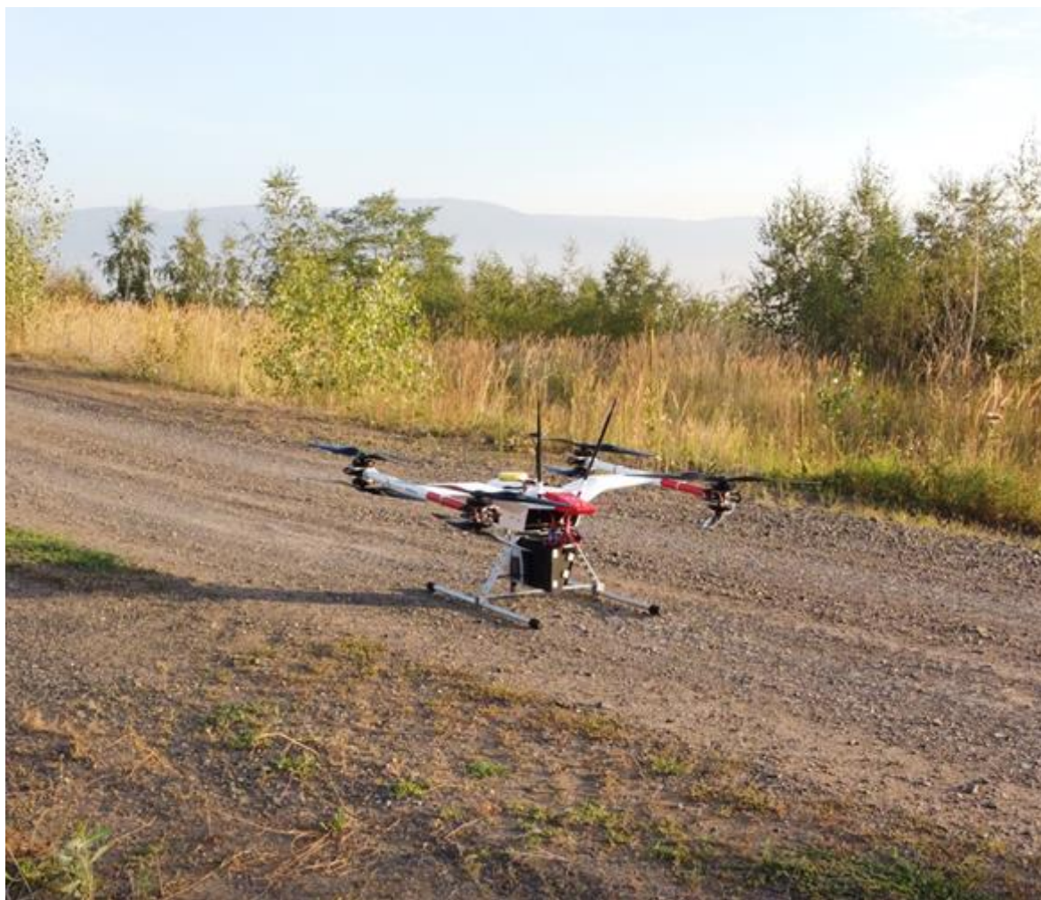
Fig. 12 Dron serving as a carrier of instruments for measuring air quality (Photo: Tušimice Observatory)
