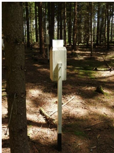
Fig. 19 “Throughfall” sampling, forest stream catchment area of the Košetice observatory (Photo: J. Svobodová)
