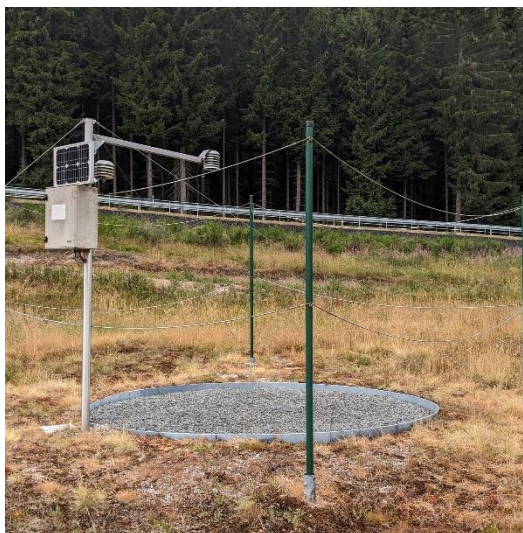
Fig. 2 Automatic snow station – snow pillow type
