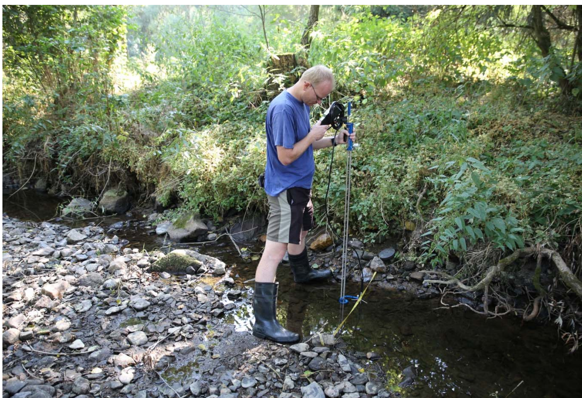
Photo 1. Discharge measurement using the flow tracker instrument at the Hrachov gauging station on the Brzina creek (7 August 2015, Lucie Petrová).
