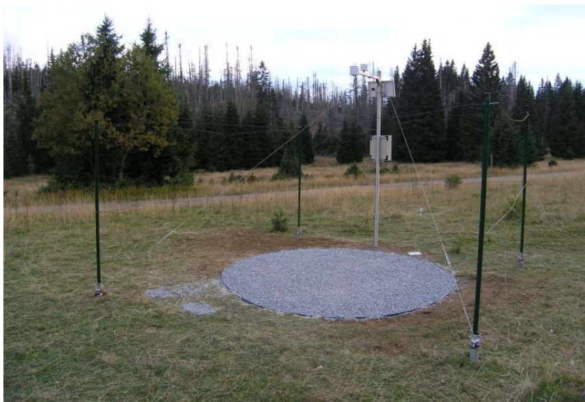
Figure P.1. Automatic snow gauging station at Javoří Pila, Šumava Mountains.
