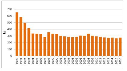
Emissions from railways are strongly dependent fuel on consumption. Emissions of GHG are given in Fig. 3-33. The sharpest decrease in emissions occurred before 1994. This was connected with a decrease in freight transport, because of significantly lower coal mining intensity compared to the period before 1989. Another factor was electrification of the core network and modernisation of rolling stock during these years. In the following years, GHG emissions increased slightly between 2004
