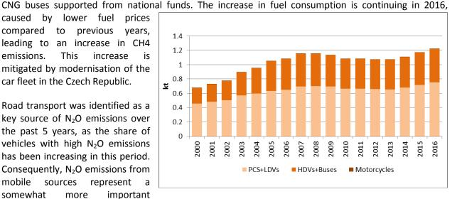
Fig. 3-31 Emissions of N<sub>2</sub>O from road transport according subsectors
