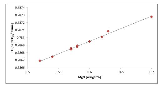
Fig. A3 6 Correlation between emission factor and mass representation of MgCO<sub>3</sub> in input material
